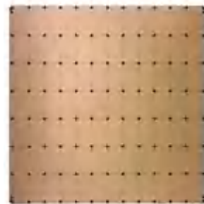
Cerebras WSE-3 4 Trillion Transistors 46,225 mm 2 Silicon
